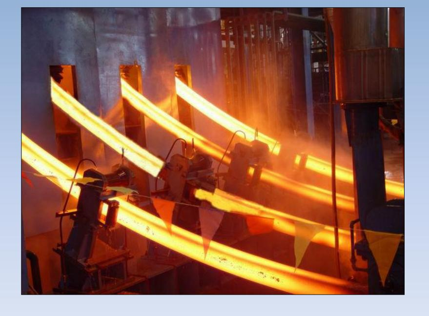
Continuous casting machines revolutionized metal processing.
